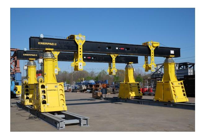
The 500-ton capacity hydraulic gantry features four legs with internal three-stage doubleacting hydraulic cylinders, octagonal boom design for added strength, fixed boom, and self-propelled steel wheels for travel on skid tracks. Each lifting tower is also equipped with a counter balance valve, stroke sensor and pressure transducers for use with the Intelli-Lift Wireless Control System.
