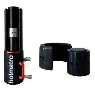
12 inches retracted, each portable, ergonomic cylinder has a lifting capacity of 100 tons but weighs only 50 pounds and features a compact footprint. Its innovative design eliminates the need for stacking wood or filler blocks and expedites the lifting process. With a stroke of 4.7 inches, the solution can safely lift and mechanically secure a load.
